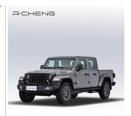
The Jeep Gladiator Overland Pickup boasts a durable and powerful 3.6-liter V6 engine that produces 285 horsepower and 260 pound-feet of torque. The engine is paired with a smooth-shifting eight-speed automatic transmission for effortless acceleration and superior fuel economy.
